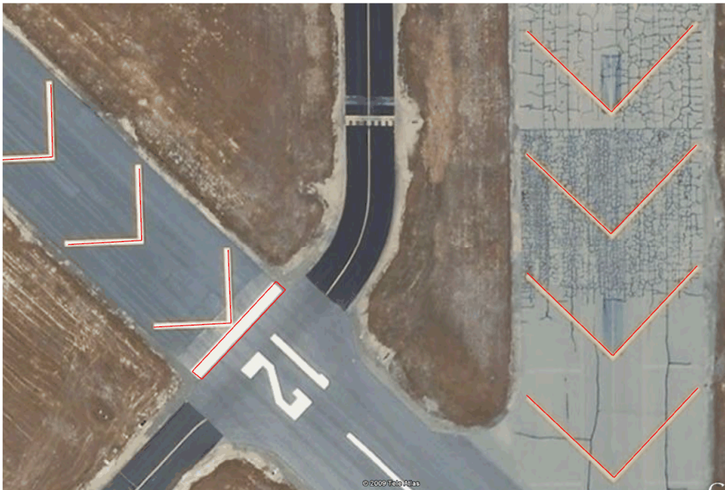
Figure viii – Red lines represent data collected in 3D using lidar generated stereopairs
