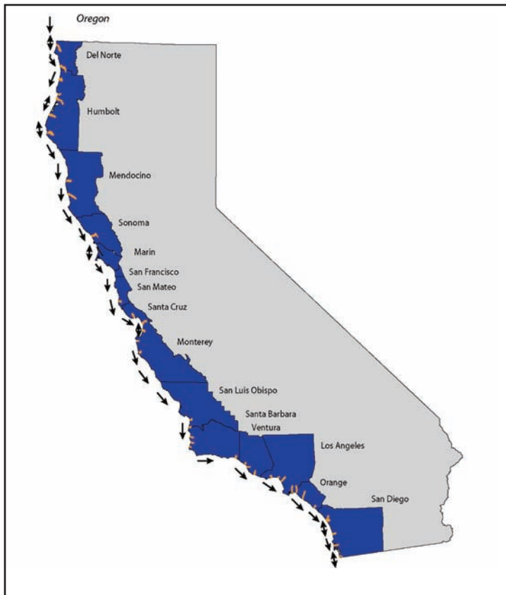
Figure 2.2: Net littoral drift directions in California
